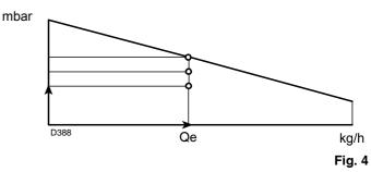
A reduction in delivery is accompanied by a reduction of the pressure in the combustion chamber:
