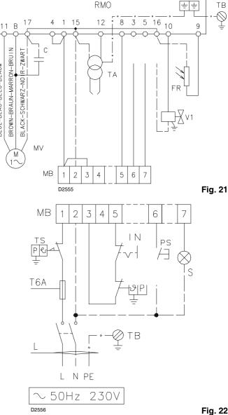
Fuse and cable sections: (cable section not indicated: 1,5 mm<sup>2</sup>)
